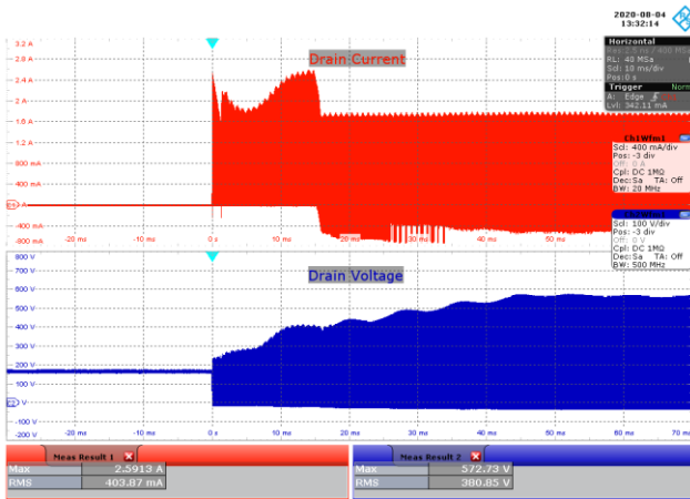
Figure 71 – 115 VAC 60 Hz, Full Load Start-up. Upper: I_{DRAIN} , 400 mA / div. Lower: V_{DRAIN} , 100 V / div., 10 ms / div.
